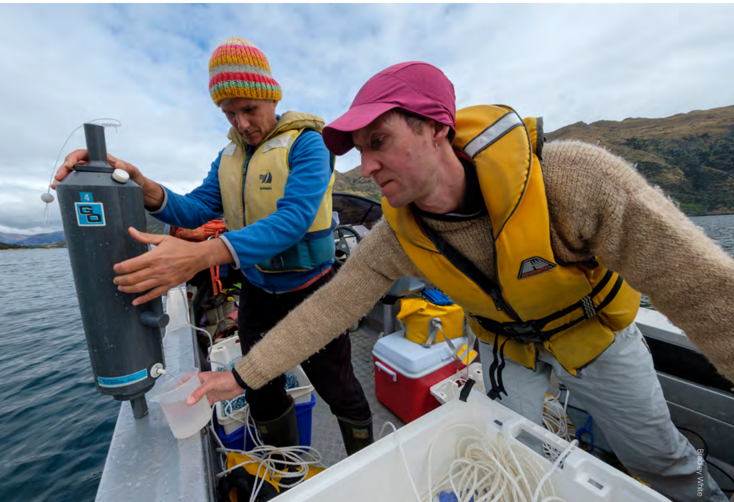
Phil Novis and Marc Schallenberg collect water from 15 m depth in Lake Wanaka, using a Van Dorn sampler. The sample contains lake snow and its causative agent, Lindavia intermedia .
